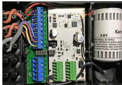
Installed LoRaWAN module inside Kamstrup MULTICAL reader
