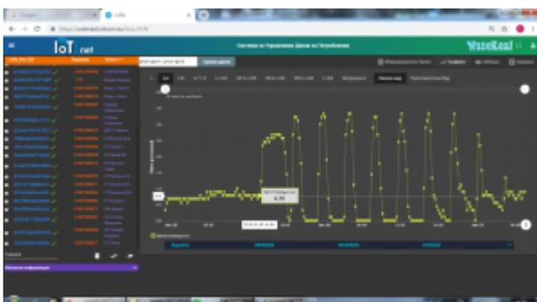
The water consumption mirrors the operational regime of the village reserved tank – the water in the network is fully utilised, following by start of the water pumps to supply water from the reserved tank, it is utilized again on the next day and again finished.
